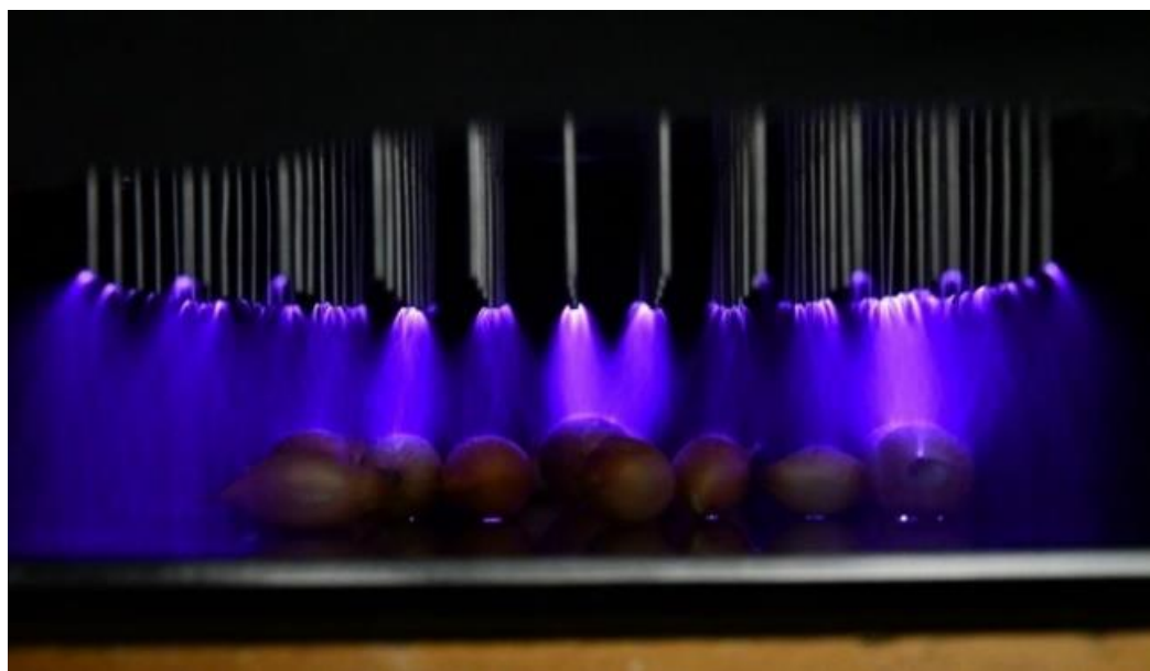
Fig. 1. Modification of bulbs by corona discharge.
