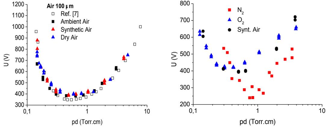
Figure 3 Comparison of the experimental Paschen curves for DC breakdown at one electrode separation a) in air, the data in [7] where measured at different electrode gap and different electrode material b) in  $\text{N}_2$ ,  $\text{O}_2$  and synthetic air
