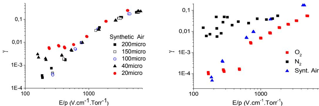
Figure 4. The second Townsend coefficient  $\gamma$  as determined from the experimental Paschen curves for a) synthetic air at different electrode separations b) in  $\text{O}_2$ ,  $\text{N}_2$  and synthetic air at electrode separation of 100  $\mu\text{m}$ .
