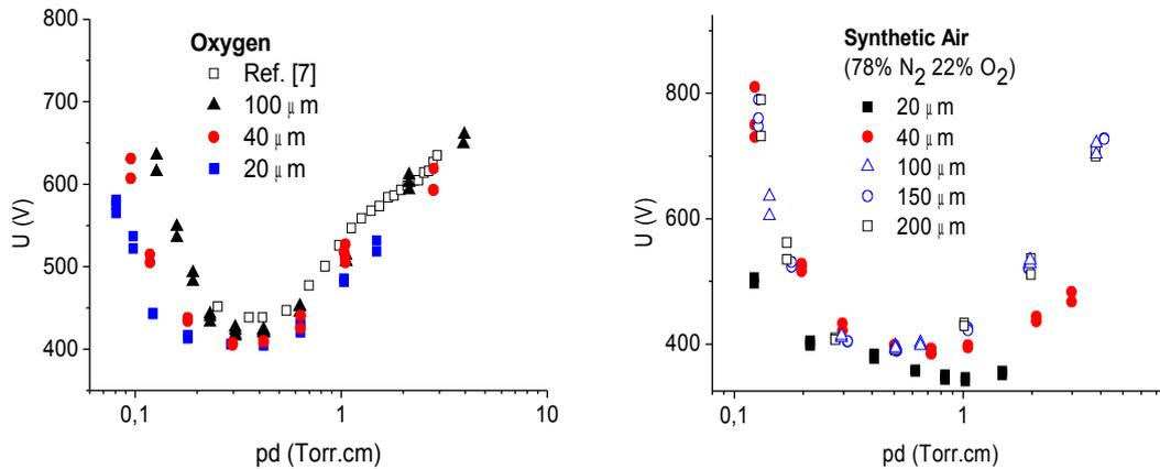
Figure 2 The experimental Paschen curve for DC breakdown for several electrode gaps a) in  $O_2$ , b) in synthetic air.
