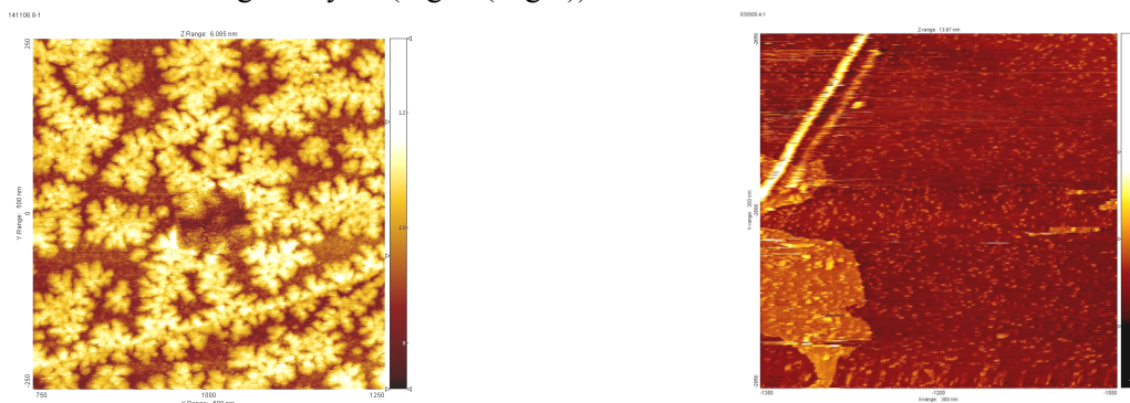
Fig. 1: Left: Fractal structure and decoration of defects; Right: Formation of silicon nanoparticle islands Modifications like vaporization, fusion and removal of nanoparticles with the STM tip on the nanometer
