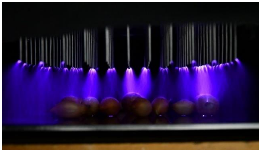
Fig. 1. Modification of bulbs by corona discharge.
