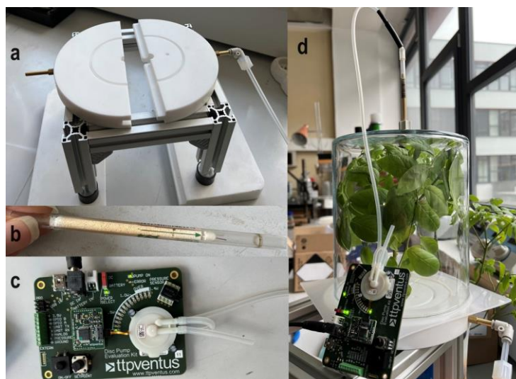
Fig. 1. Experimental setup for collecting the emitted VOCs from blueberry leaves including (a) a Teflon guillotine-like base, (b) Tenax trap as an adsorbent, (c), a small pump and (d) the final assembled setup including a glass cylinder and a blueberry branch in it.
